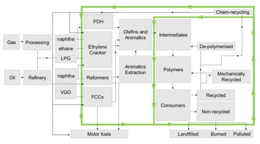
Depolymerization is another recycling technology that allows for waste feed streams to be converted into their pure monomers. The most common
